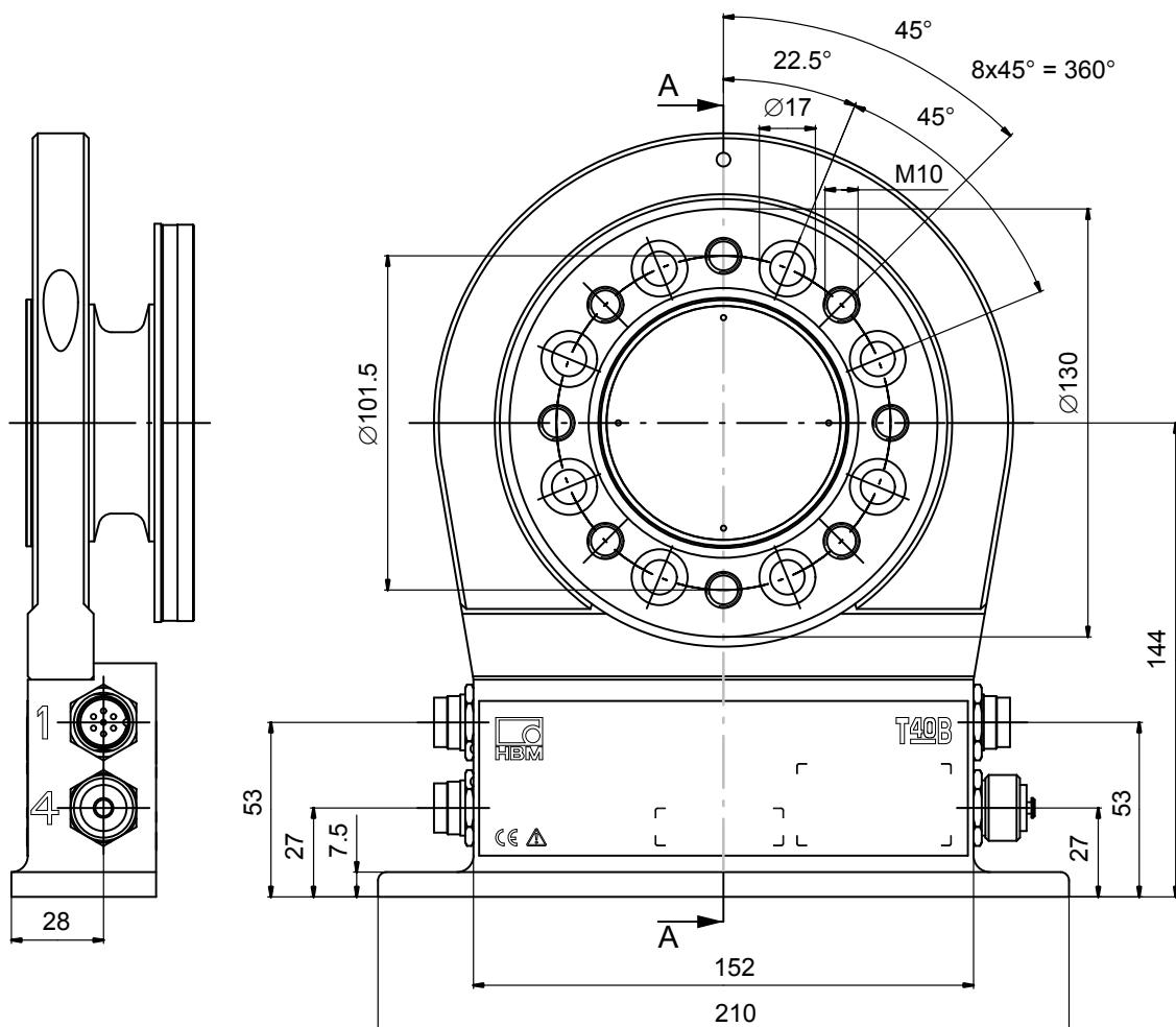
**Dimensions of T40B/500 Nm and 1 kNm without rotational speed measurement, continued**
