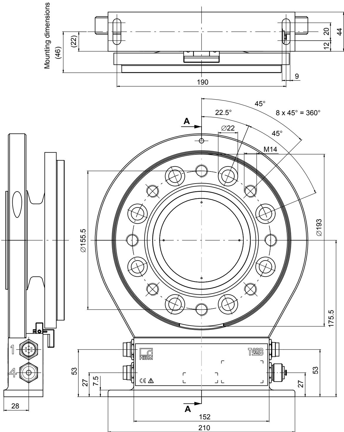
**Dimensions of T40B/5 kNm with rotational speed measurement and reference signal,
