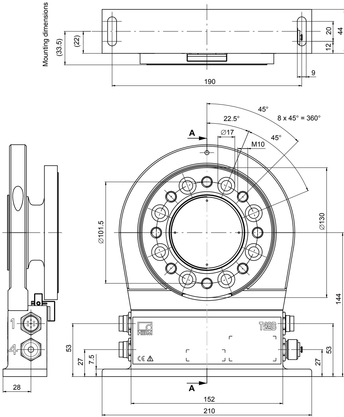
**Dimensions of T40B/500 Nm and 1 kNm with rotational speed measurement and reference signal, continued**
