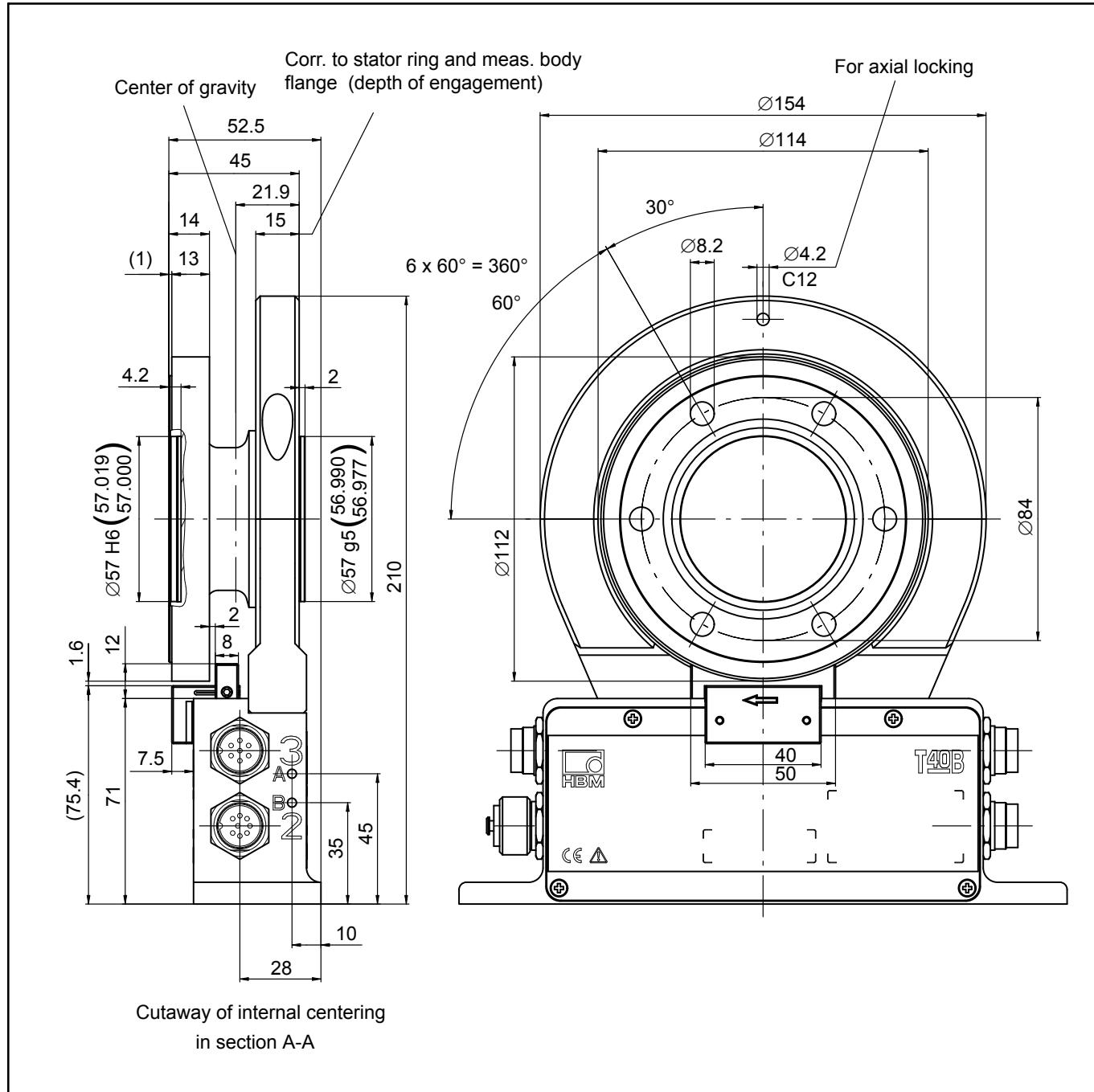
**Dimensions of T40B/500 Nm and 1 kNm with rotational speed measurement and reference signal**
