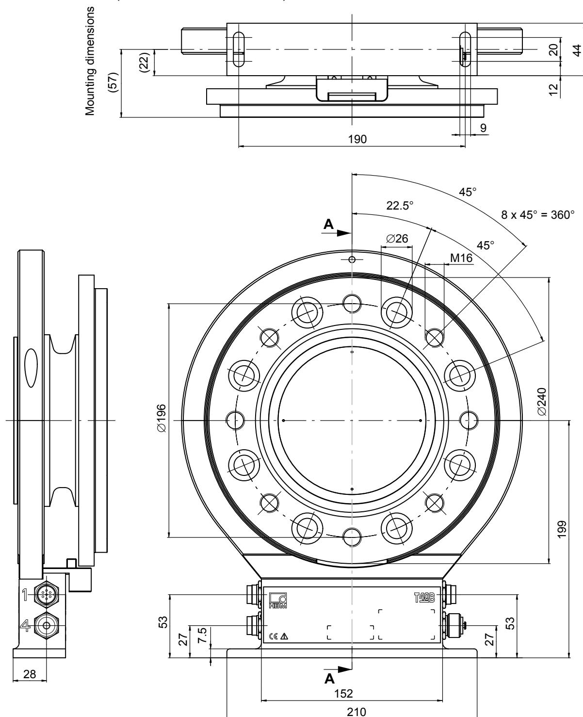
**Dimensions of T40B/10 kNm with rotational speed measurement and reference signal,
